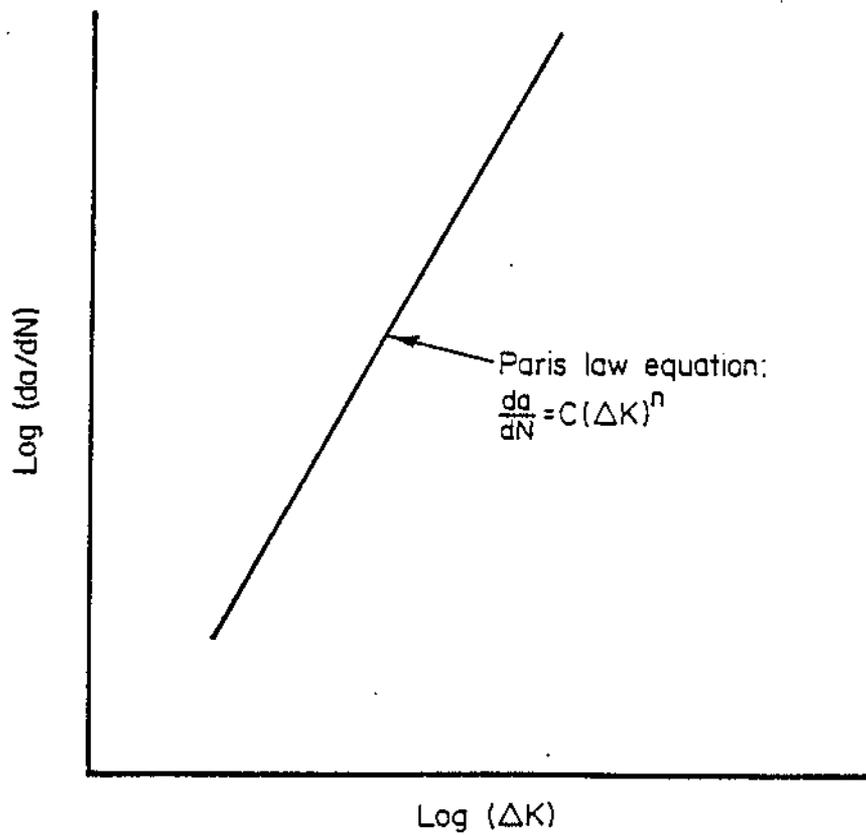
**Figure 4. Typical Plot of Fatigue-Crack-Growth Rate (da/dN) Versus Change in Stress-Intensity Factor (Δk) on Log-log Coordinates Showing Paris Law Fit of the Data**
