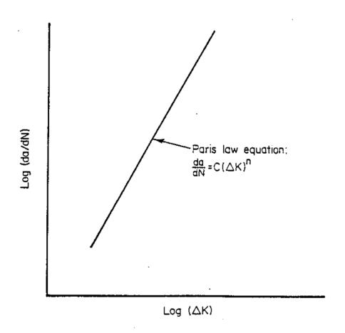
Figure 4. Typical Plot of Fatigue-Crack-Growth Rate (da/dN) Versus Change in Stress-Intensity Factor ( $\Delta k$ ) on Log-log Coordinates Showing Paris Law Fit of the Data
