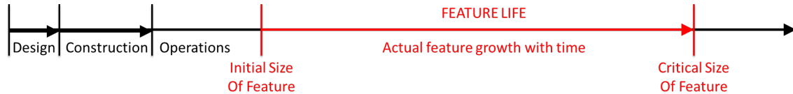
Figure 12. Timeline Showing Feature Life from Time of First Initiation with Feature Growth Until the Feature's Critical Size is Reached.
