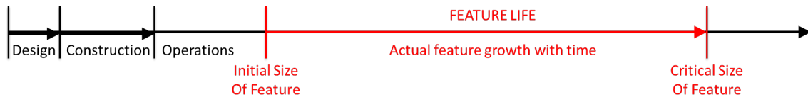
Figure 2. Timeline Showing Feature Life from the Time of First Initiation with Feature Growth Until the Feature's Critical Size is Reached
